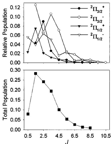
FIG. 5. OH photofragment distributions resulting from photodissociation of  $\text{H}_2\text{O}(|02\rangle^-)$  in  $2_{02}$  rotational state plotted as a function of  $J_{\text{OH}}$ . While the populations within the individual spin-orbit and  $\Lambda$ -doublet manifolds (top panel) strongly oscillate with  $J_{\text{OH}}$ , the total population (bottom panel) is much smoother reflecting the interference nature of the photodissociation.
