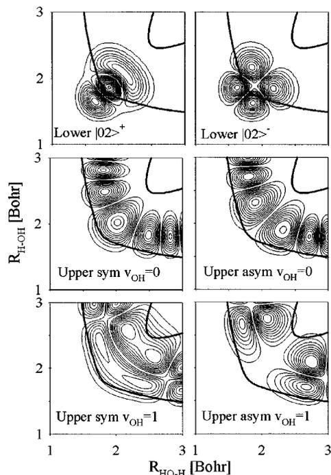
FIG. 10. Ground state ( $|02\rangle^+$  and  $|02\rangle^-$ ) and excited state symmetric/antisymmetric wave functions correlating with  $\text{OH}(v=0,1)$  and accessed via excitation near 193 nm. Bold lines surround the energetically accessible Franck–Condon region for 193 nm excitation out of  $v_{\text{OH}}=2$  H<sub>2</sub>O states. Contours corresponding to positive and negative wave function values are shown in solid and dashed lines, respectively.
