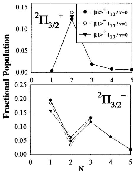
FIG. 3. A subset of relative OH( $v=1$ ) and OH( $v=0$ ) populations in  $2\Pi_{3/2}^{\pm}$  manifolds resulting from UV photolysis of  $|02\rangle^{+1}_{10}$  and  $|11\rangle^{+1}_{10}$  states of H<sub>2</sub>O. Strong similarities in the observed distributions support the assumption of decoupling between vibrational and rotational degrees of freedom in OH photofragments (this assumption is used to derive relative final vibrational populations of OH listed in Table I).
