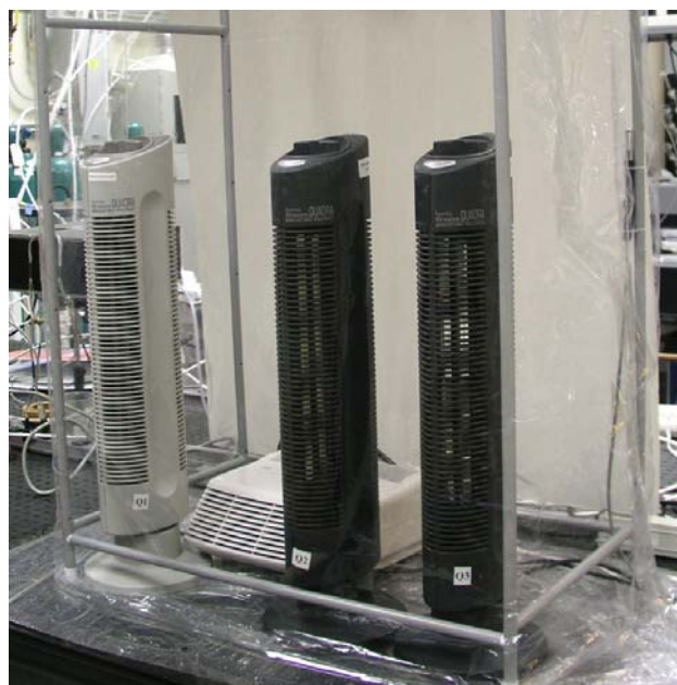
Figure 1a: Schematic diagram of a possible fixed-volume chamber design for this project and a photograph of an actual chamber with several air purifiers inside. The aluminum frame visible in the photo comes from an Ikea wardrobe. The Teflon film is thermally sealed on top and all sides of the frame. Loose ends of the Teflon film at the bottom are attached to another sheet of Teflon film on the table surface with tape.
