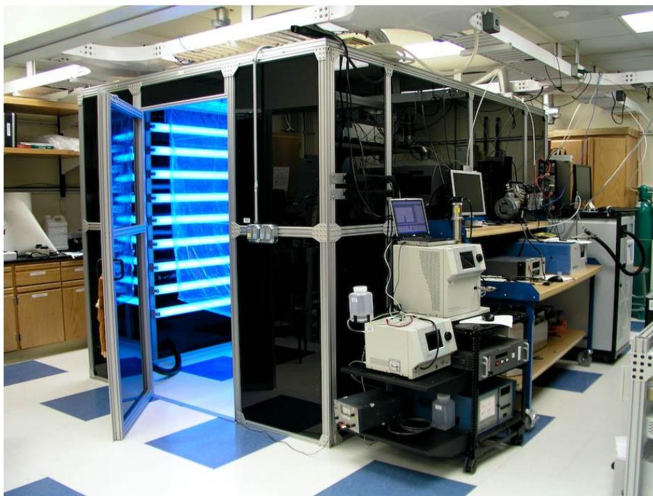
**Figure 1.5:** Picture of the UCI Photochemical Chamber with UV-B lights turned on.
