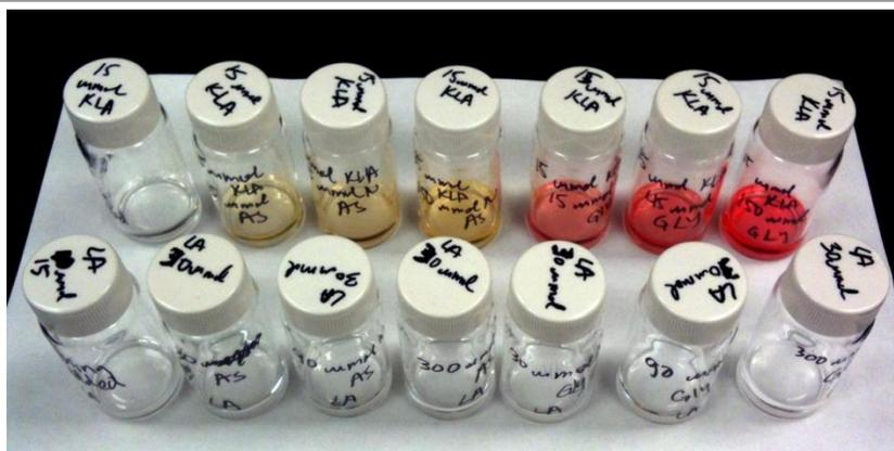
**Figure 8.4.** KLA aqueous solutions (top row) form visible light-absorbing chromophores from addition of ammonium sulfate (AS) and glycine (GLY) while LA solutions (bottom row) do not. Top row from left to right: KLA (control), AS/KLA (1:1), AS/KLA (3:1), AS/KLA (10:1), GLY/KLA (1:1), GLY/KLA (3:1), GLY/KLA (10:1). Bottom row: same AS and GLY ratios as top row but with LA instead of KLA.
